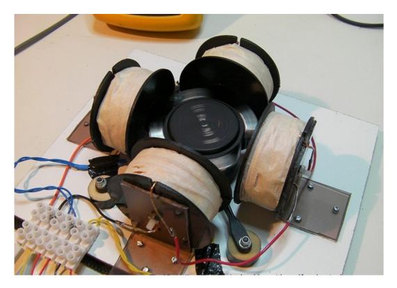
The "Brandon motor" uses four AIR CORE coils and four NdFeB magnets mounted on rotor.
