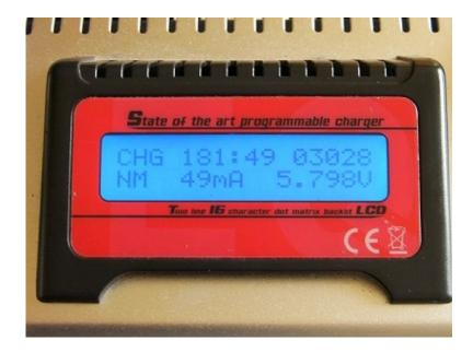
After the long week test run in closed loop, the NiMh battery has been recharged and 3028 mA have been reloaded.
