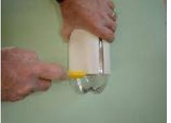
100 mm: 1 to 29 cm and the other with 31 cm and then make a cut lengthwise in 2 tubes, allowing the placing the bottle in it, defining the size of the cylinder to be cut. The pipe of 29 cm used for measuring the cutting of Lisas and bottles of Pepsi (new model) and the tube of 31 cm only for the cutting of bottles of Coke.
