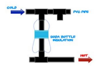
The standard solar water heaters cost a couple of 1000\$ and have copper as a main element. The Plastic Bottle solar water heater cost almost 50 \$ and is based on the thermosyphon technology which is used in many solar water heaters. It makes use of the circulation of water based on density; hot water which is less dense moves upwards while the cold water which is denser moves down. As long as the possibility of installation of the collector
