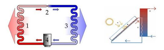
with the top of the same, ie the top bar the return of hot water, be between 10cm. and up to 3 meters below the lower (bottom) of the housing or shell, as the diagram below.
