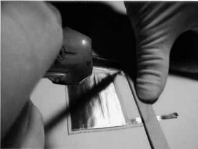
Sealing plastic with solder-iron
