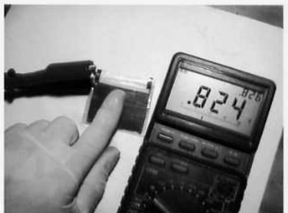
Two cells measures .824 vDC
