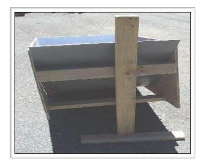
The photo above shows the back side of the cooker, where the 2x4 spreaders can be seen. Note also the remaining length of 2x4 is used as a support (more about that later).
