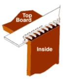
You can then join the boards together at the joints securing with glue and clamping overnight.
