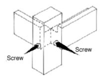
Ideally, the side supports should be attached at even intervals (every 30"), but you can modify this to suit your own requirements. Repeat for the other side, taking care to ensure that the routed groove points towards the middle of the shelving unit. Take the time to ensure that all joints are square; otherwise you may end up with a shelving unit that leans!
