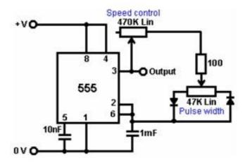
As this allows the speed to be controlled and when the required speed is reached, the pulse width can then be adjusted to give the minimum current draw to maintain that speed. There are, of course, many other suitable circuits which could be used instead of this one and Chapter 12 will fill you in on some of them as well as explaining how circuits work and how to build them.
