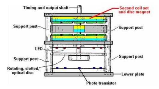
The coil switching with the additional layer of coils is shown here:
