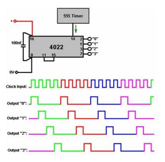
The output voltage on the pins marked "1", "2", "3" and "4" goes high one after the other as shown in the diagram above. So, each of these output pins would be connected to the FET gates in that order and the FETs would get switched on in that same order.
