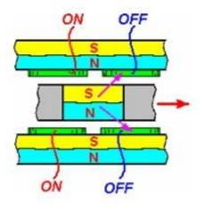
This produces a larger horizontal thrust. While this design goes for optimum performance, I suggest that a much more simple form of construction with a ring of standard circular neodymium magnets could be used instead of one large disc magnet, and ordinary circular coils placed on top of the circular magnets, and this allows large diameter rotors to be constructed, the larger diameter giving greater output shaft power:
