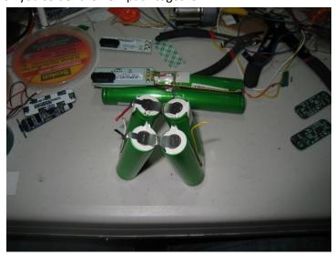
This is the pack, folded in half in the middle. I cut the tabs in such a way to leave each battery enough tab to fold back over itself. This is important, because you cannot solder directly to a cell end, but you can solder to the tab attached to it.
